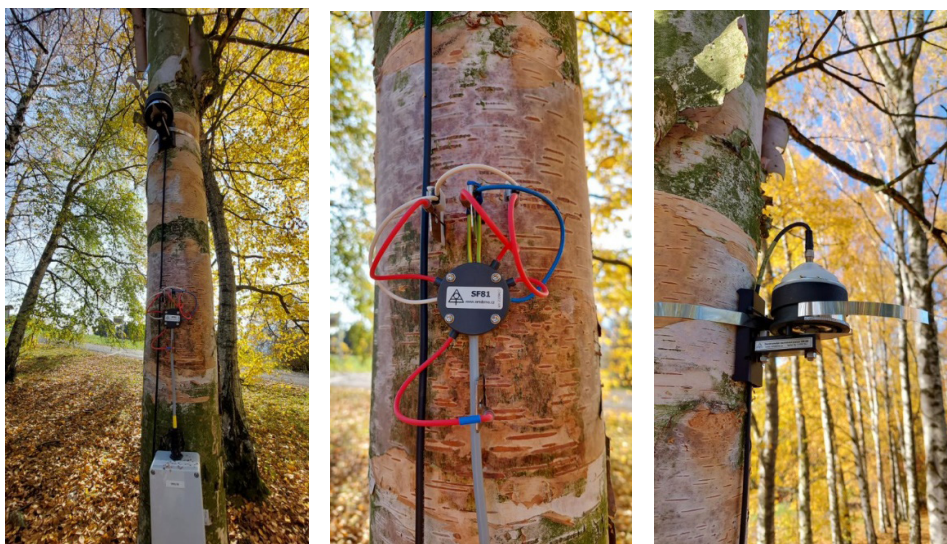
Fig. 5 Installed Sap flow System in combination with measurement of tree trunk circumference changes and increment
